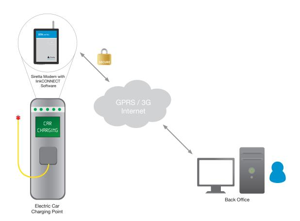
GSM also offers multiple options for connectivity, such as, sending data over GPRS, CSD or via SMS, ensuring that you can connect one way or another.
