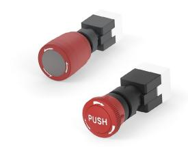
TE Connectivity (TE)'s ALCOSWITCH PBES16 Series Pushbutton Emergency Stop Switch is offered as an illuminated and non-illuminated switch. This series has multiple lighting options, agency approvals, and meets IEC 60947-5-1 and IEC 60947-5-5 standards. These switches are offered with two different actuator button styles. The PBES16 Series has a 20N actuation force for ruggedized applications to avoid accidental actuations and is also IP65 rated to withstand harsh environments.
