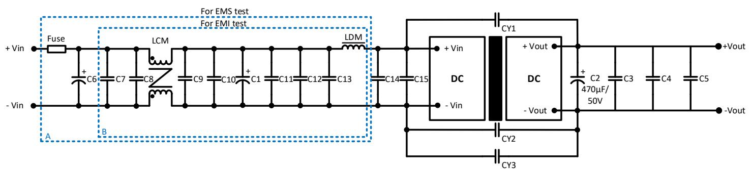
Notes: Part A for EMS filtering and Part B is used for EMI filtering.
