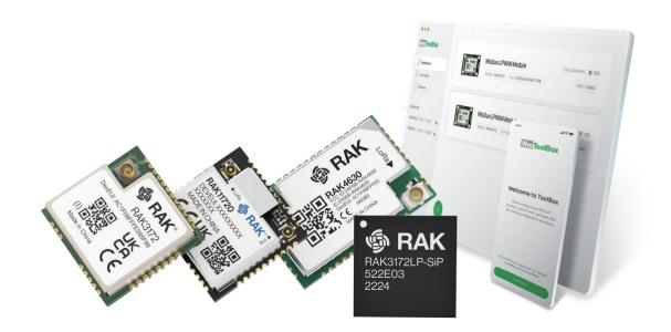
The modules integrate both a microcontroller and a LoRa® transceiver in a compact format. Compliant with LoRaWAN® 1.0.3 protocols, they ensure a seamless connection with an external MCU through a simple AT command interface. Furthermore, these modules allow for hosting the application directly, making them capable of both communicating via LoRa and functioning as an MCU.
